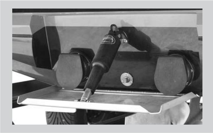
The wake plate allows the driver to control the running attitude of the boat. It can be controlled by the switch on the dashboard.
