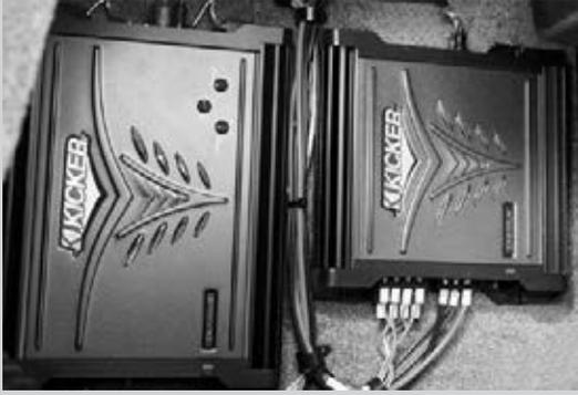
The stereo amplifier is an optional piece of stereo equipment that is designed to increase the wattage of the signal going to the speakers while minimizing distortion of this signal. Please see stereo amplifier owner's manual for more information.
