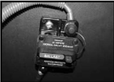
The power to the ballast pump circuit is protected by a circuit breaker that is located in the port side of the engine compartment.
