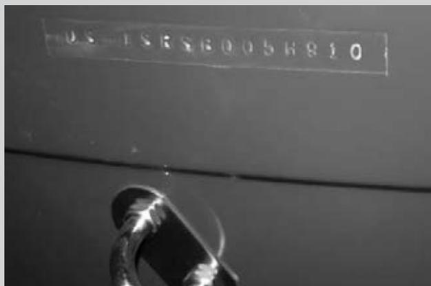
The hull identification number is located on the upper right hand side of the transom below the rub rail.
