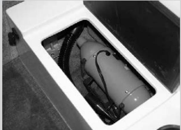
The models with steps come standard with an air inflator. It is a high volume, low pressure pump designed specifically for tubes, air mattresses, etc. To use the pump, pull the unit out of its storage compartment located to the rear of the walk through area and plug the cord into the 12 volt receptacle. Connect the hose of the inflator to air input on inflatable object and turn on.
