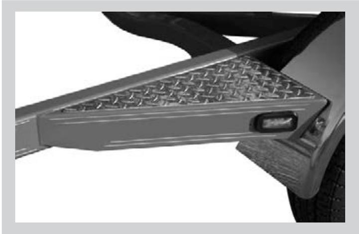
The optional aluminum step plate gives the trailer a durable, long-lasting nonskid surface on the trailer steps.
