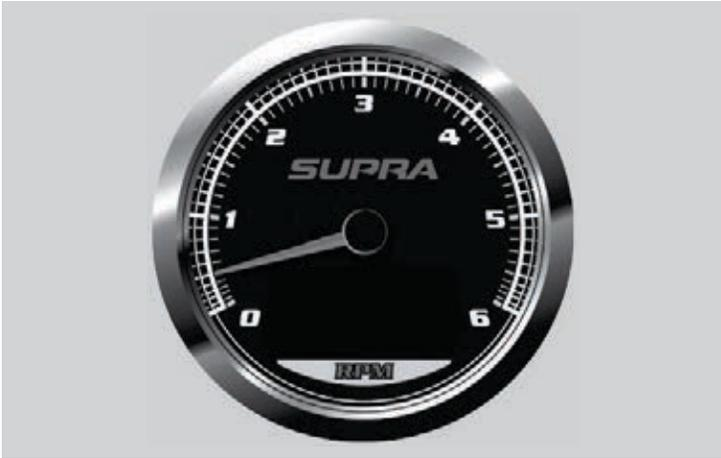
The tachometer indicates the engine revolutions per minute (RPM).
