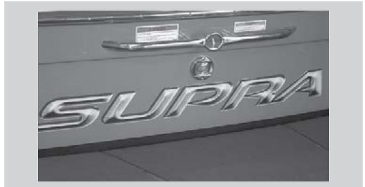
Some Supra models are equipped with stern lights. The stern light is located at the center of the transom below the rub rail. The stern light is activated by the "Courtesy" light switch.
