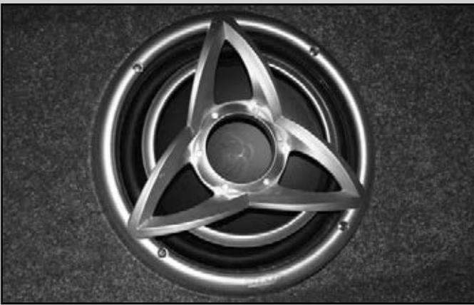
The optional subwoofer is designed to increase the sound level of the bass notes. The amplifier powers the subwoofer. The bass level can be adjusted on the amplifier. Please see stereo amplifier owner's manual for more information.
