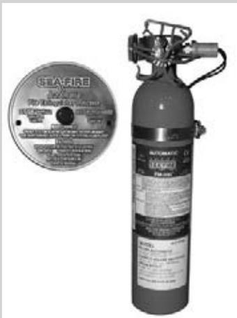
The optional Automatic Fire Suppression System has a sensor in the engine compartment that is designed to detect a fire. Under normal conditions, the dash area warning light will glow green when the ignition is "ON". If the engine compartment sensor is activated by a fire, it will deploy the content of its fire extinguisher and the dash mounted warning light will turn red.
