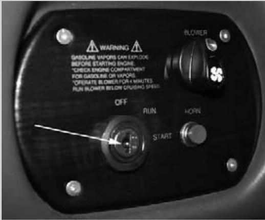
Located on the port side of the dashboard, the ignition switch has four positions. In the vertical position the ignition is "OFF". In the OFF position, only the blower and bilge switches are powered.
