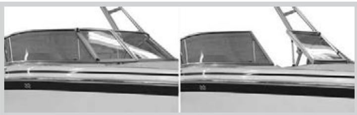
The movable center windshield panel allows access to and from the bow deck. To open, turn safety latches to vertical and push. Lay the center windshield panel gently against the fixed side panel.
