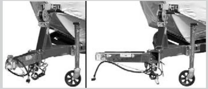
With the swing tongue, you can shorten the trailer length for storage by pulling the pin and swinging the tongue away to the side.
