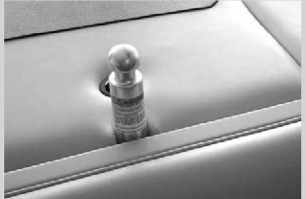
The ski pylon is to be used to pull skiers. DO NOT use ski pylon to hoist boat! Only use the lifting rings for this purpose.
