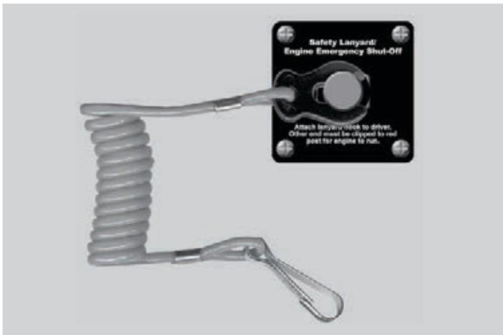
Your Supra is equipped with a Safety Lanyard/Engine Shut Off switch. In order for the engine to run, the plastic tip of the safety lanyard must be attached to the switch. If the clip is removed from the switch, the engine will not run.
