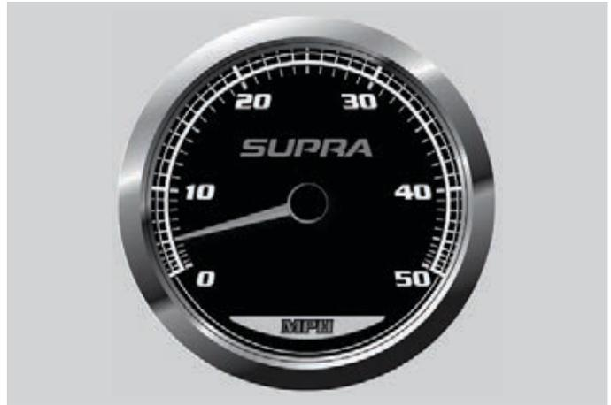
The speedometer indicates the water speed of the boat in miles per hour. It is recommended that the speedometer be checked for accuracy periodically.
