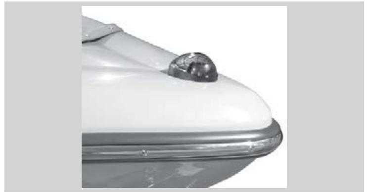
The bow light is located on the bow of the deck at the front of the boat. To alert other boaters to your position and direction, the light is green on the starboard side and red on the port side. The bow light is activated by the "NAV" switch.
