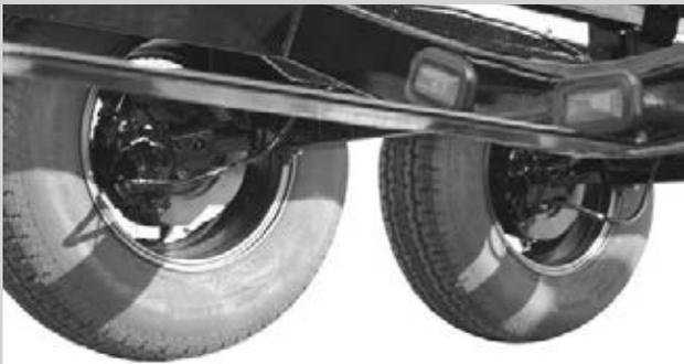
The second axle disc brakes give the trailer more stopping power.
