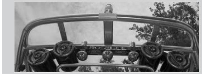
The optional tower speaker and light bar combo is a unit that houses both an additional set of tower speakers and lights. The speakers are designed to allow the rider to be able to hear the music. The tower speakers require the addition of an amplifier to power the speakers. The tower lights are designed to make docking, loading and unloading easier. The tower lights require the addition of a dual-battery electrical system.
