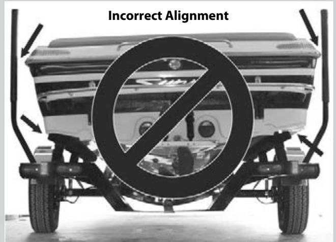
The distance between the boat and the wheel runner board should be equal on both sides.
