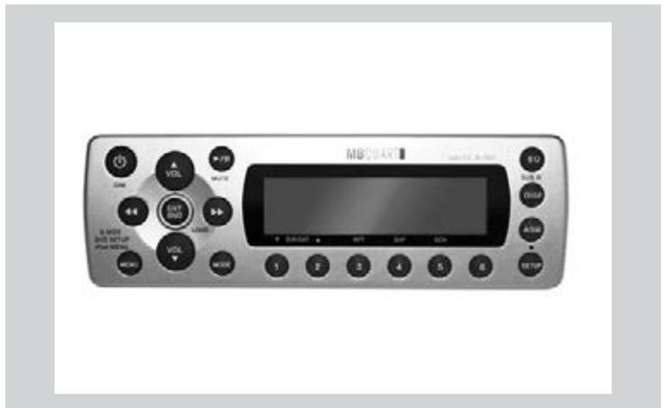
The optional transom mounted stereo remote allows the stereo to be controlled from the rear of the boat.
