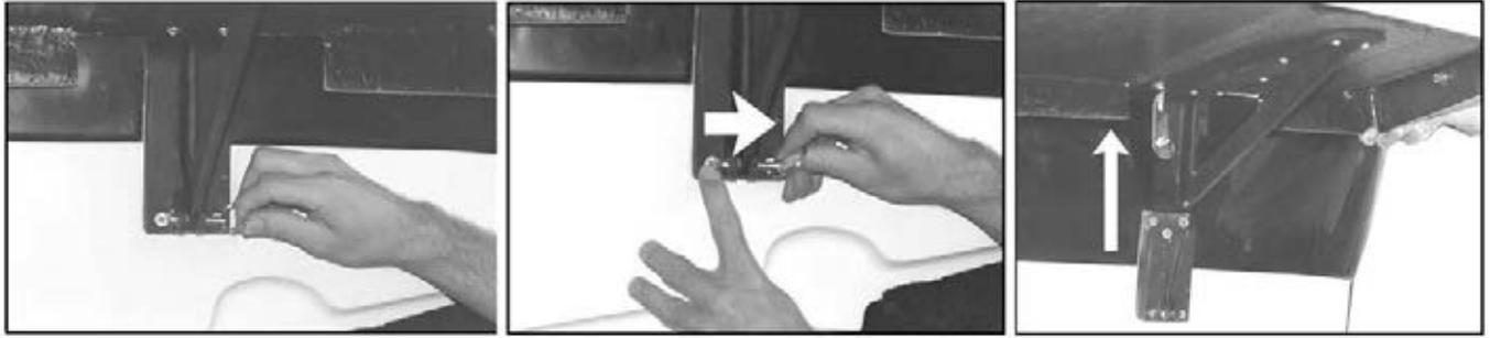
The ski platform is attached to the boat with detachable brackets. The platform may be removed from the boat by pulling the retaining pins from the brackets and lifting up and out.
