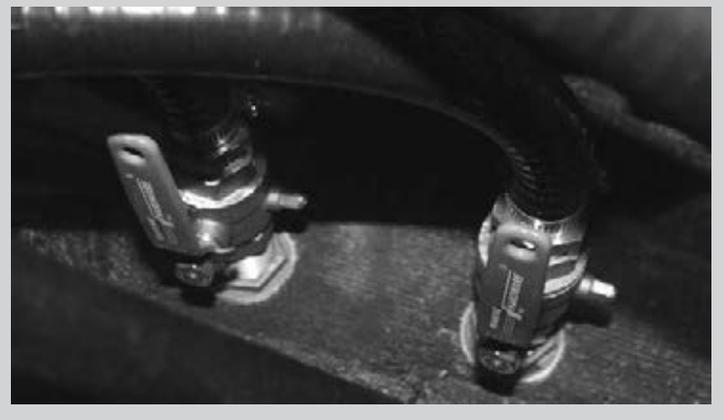
Each Gravity Ballast System also includes manual shut off valves in case of emergencies. If closed, the valve will prevent any water from entering the system and is only used in emergency situations. Under normal use the valve should remain open to allow full flow of water into the system.
