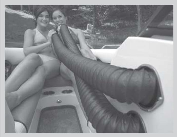
The boat heater is a forced air heater that uses hot engine water as a heat source. To use the heater, simply turn the heater switch to the selected fan speed. In order for the heater to work, the engine must be at operating temperature. One of the features of the heater are the snorkel vents, which can be pulled out to direct heat to specific areas.
