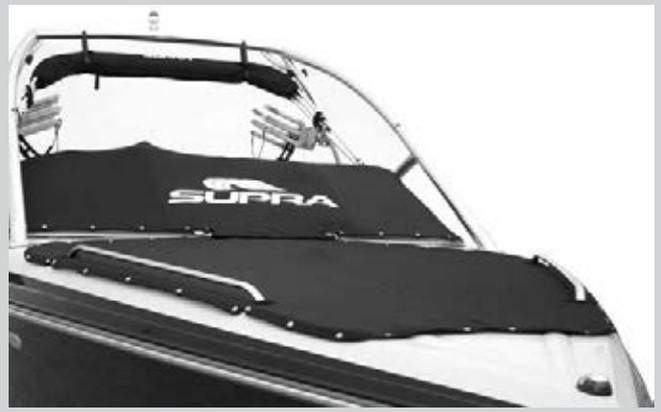
The optional tonneau cover is designed to snap over the bow of the boat. Its purpose is to minimize air flow into the cockpit area when the boat is in use and as a storage cover when used in combination with the optional cockpit cover.
