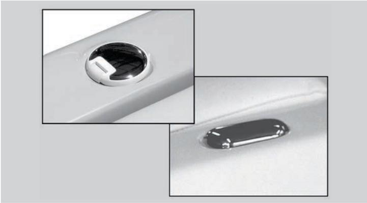
The pole light receptacle is located on the starboard of the stern, along side of the sun deck. To install pole light, slide open the weather cover and insert the pole light in the aligned position.
