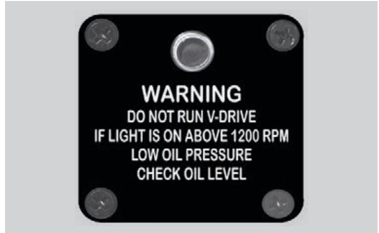
The V-Drive transmission in your Supra is equipped with a "low pressure" warning light. This light is located by the dash. Do not operate your Supra if the warning light remains on, whenever the engine speed is above, 1,200 RPM (+/- 400 RPM). This warning light should be on whenever the engine speed is below 1,200 RPM (+/- 400 RPM). If this light remains on during operation above idle, shut your engine off immediately and check your v-drive oil level and see your dealer.
