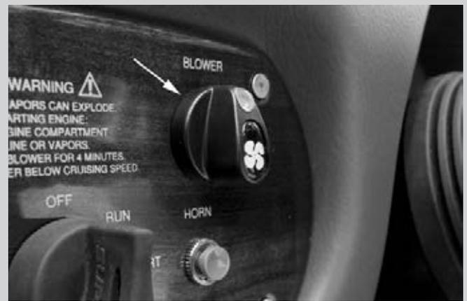
The blower switch activates the blower motor. The primary function of the blower fan is to remove any fumes from the bilge area. The blower also draws fresh air into the engine compartment.
