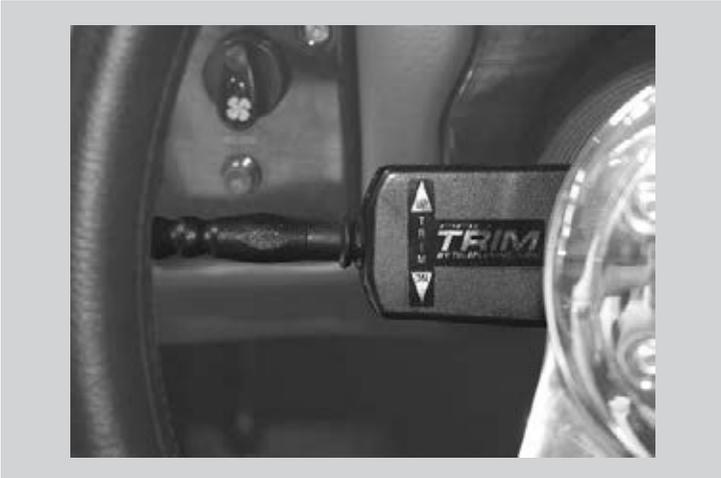
This switch controls the wake plate. The gauge indicates the position of the plate.
