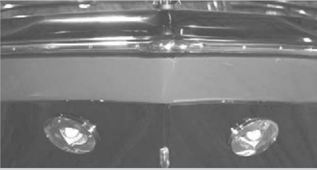
The docking lights are designed to help you dock, load and unload your boat in low light or at night.
