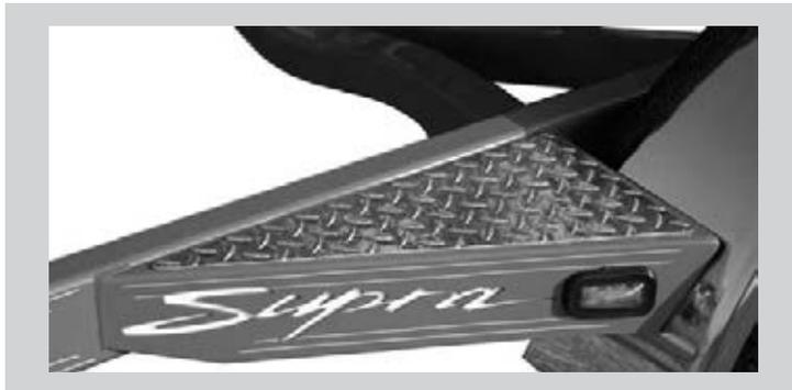
The optional laser cut steps are backlit, so they illuminate when the trailer's running lights are illuminated.
