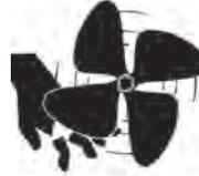
A moving propeller will cause injury. The propeller may turn with the boat in neutral. Shut off the engine while skiers or swimmers are in the water near the ski platform.
