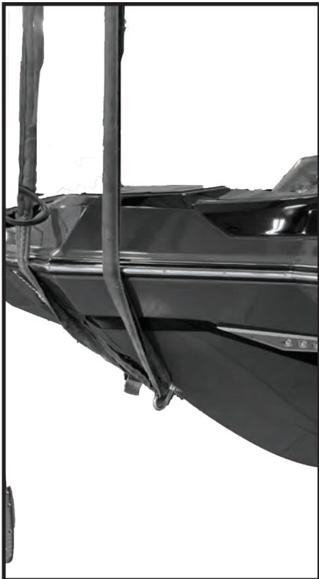
**NOTE:** For boat houses, we highly recommend the use of a lifting cradle. Cradle bunk design should mimic the bunk design of the trailer.
