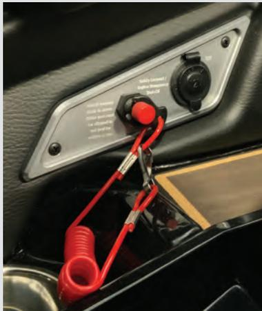
Your Supra is equipped with a Safety Lanyard/Engine Shut Off switch. In order for the engine to run, the plastic tip of the safety lanyard must be attached to the switch. If the clip is removed from the switch, the engine will not run.
