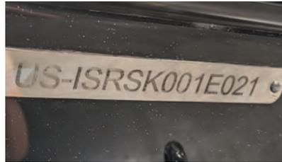
The hull identification number is located on the upper right hand side of the transom below the rub rail.
