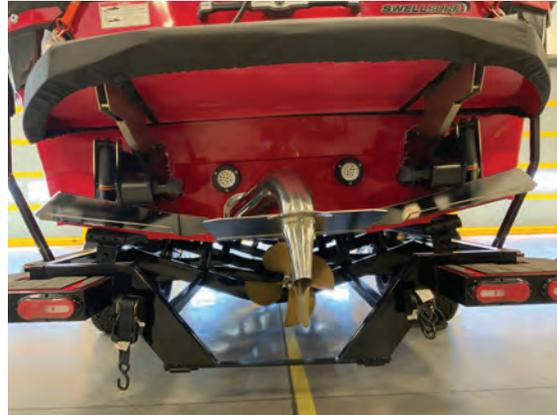
The distance between the boat and the wheel runner board should be equal on both sides.
