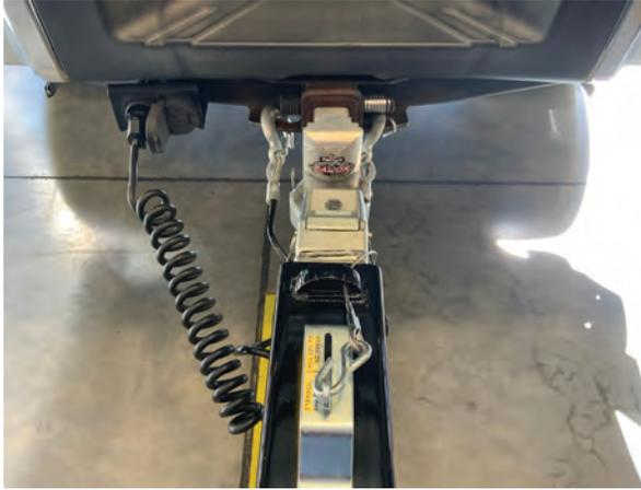
**NOTICE: If your hitch ball has an excessive flat spot on top, the latch may not engage properly. If the latch does not catch, check with your dealer or hitch installer before trailering.**
