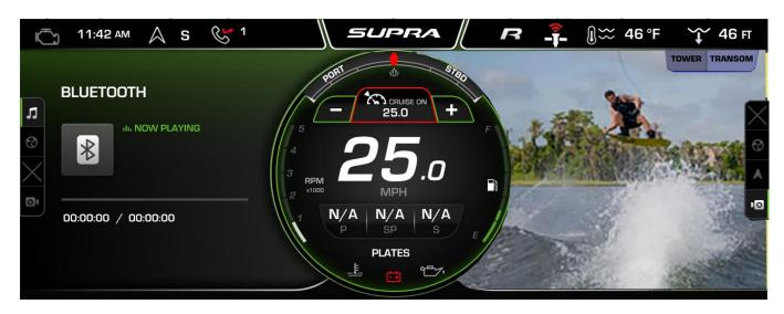
Touch the Tower or Transom button to switch to the alternate video view. Both the Tower and Transon camera video feeds will be displayed automatically when the shifter is moved to Reverse and remain on for 10 seconds when the shifter is returned to the Neutral or Forward
