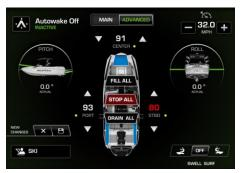
Note: The engine must be running to fill the ballast. When AutoWake is off adjust the Ballast settings by the up and down arrows.
