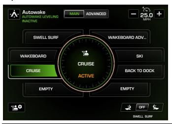
AutoWake\* is a patented system that will manipulate the ballast levels in order to achieve and maintain the best possible wake for surfing and wakeboarding. Using an inclinometer (a device that measures angle of pitch and roll) the boat will orient itself for the best boating experience.
