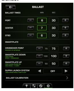
The first section of this page controls how quickly the ballast fills and drains. Use the – and + buttons to establish the minutes and seconds for the Port, Center and Starboard ballast bags.
