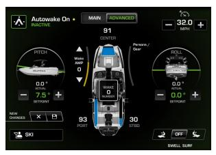
Adjust the Pitch and Roll setpoints by touching the – or + buttons. Changing these or the Wake Amp (described on the next page) will briefly display a graphic at the top of the screen illustrating the expected wave using the new settings.
