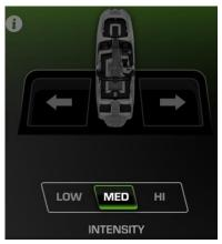
There are five states to the system: Off, Port Dock Hold, Starboard Dock Hold, Port Burst and Starboard Burst.
