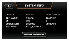
Like the System Information screen in the PV100, this screen provides version and part numbers for the Application, Operating System, Bootloader and Software, along with a method to update the software.
